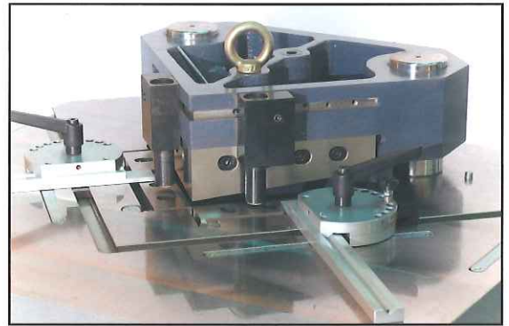
STURDY WORKHEAD, CONICAL GROOVES WITH SET OF GONIOMETRY SQUARES ON RIGID CAST IRON WORKTABLE.
